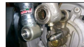
Center the pin of the HTC kit at the central hole of the wheel, and put the pins of the wheel at the beginning.
